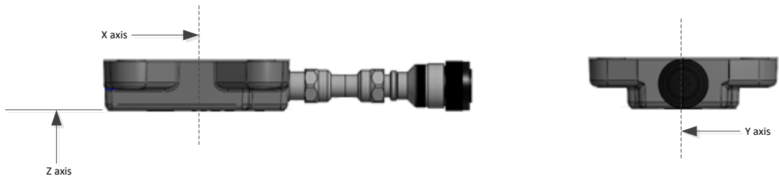
Figure 2: APC receiver reference axes
